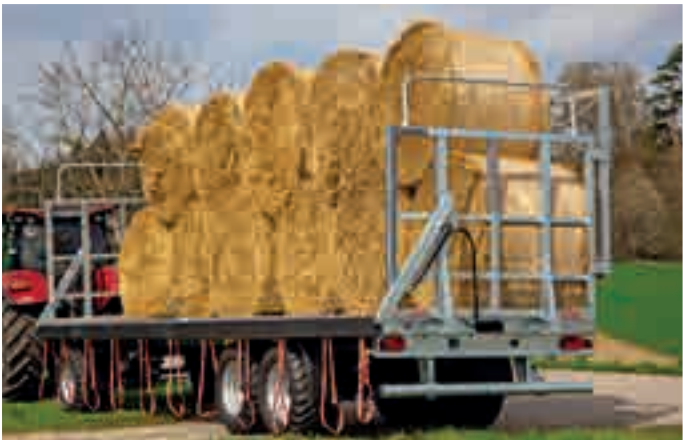
DPW 210 Ultra with open load securing
