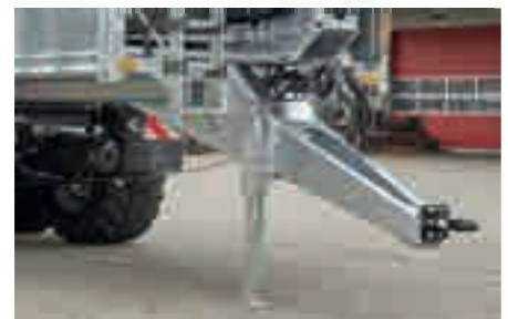
Drawbar unsprung, rotatable for Top and bottom attachment
