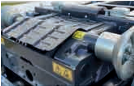
Large cast steel rollers (ø 310mm) with large centring bevel make it easier to raise the container.
