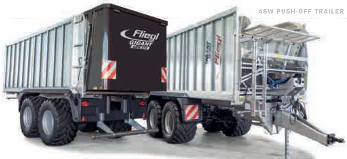
The Fliegl movable axle mechanically or hydraulic (ASW 271)
