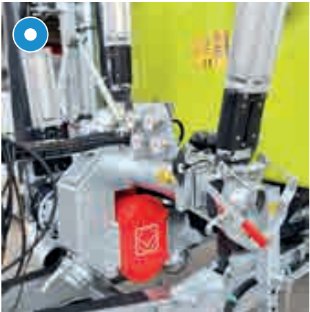
Maintenance-friendly "PolyFant" rotary lobe pump
