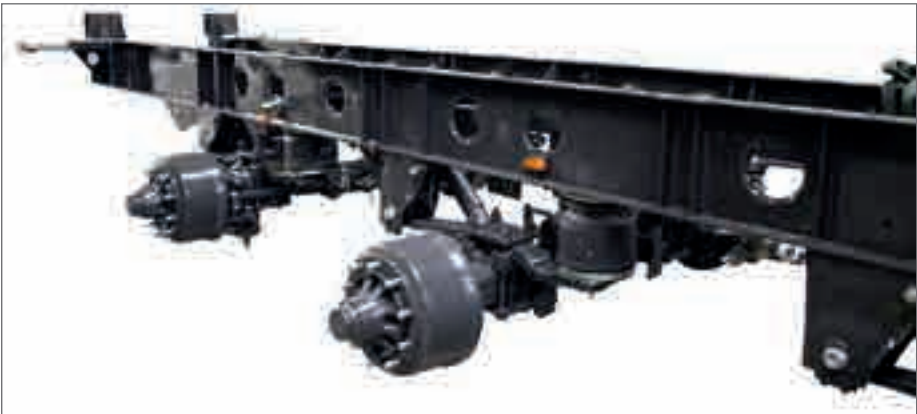
Special frame construction made from fine-grain steel
