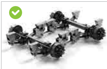
Jumbo Gigant Plus tandem assembly for 15,500 l and 18,500 l Poly Line Plus
