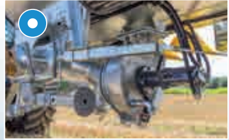
For vacuum tank: turbo filler positioned centrally under tank – for suction on either side
