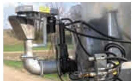
Hydraulic pendulum spreader with working width from 12 to 18 m.
