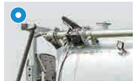
Purge line incl. three-valve for optimum stirring function
