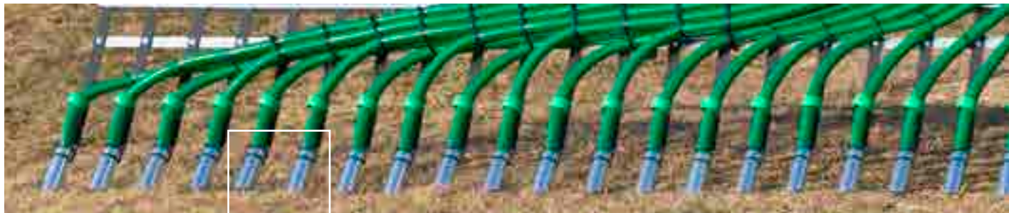
Shoe spacing of just 187,5 mm
