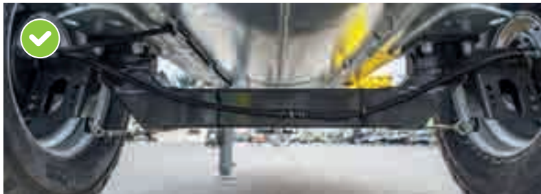
Cranked axle on 5000 to 8600 l models Low centre of gravity ensures optimum handling on slopes
