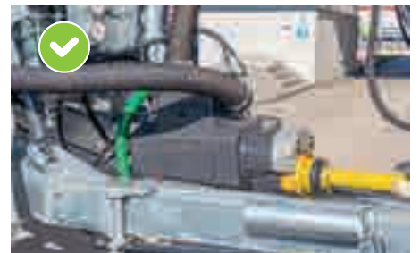
✓ Heat-resistant compressor Optional: water-cooled compressor
