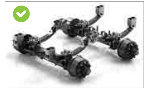
Gigant tandem assembly for 11,000 l, 12,500 l and 14,000 l Poly Line Plus
