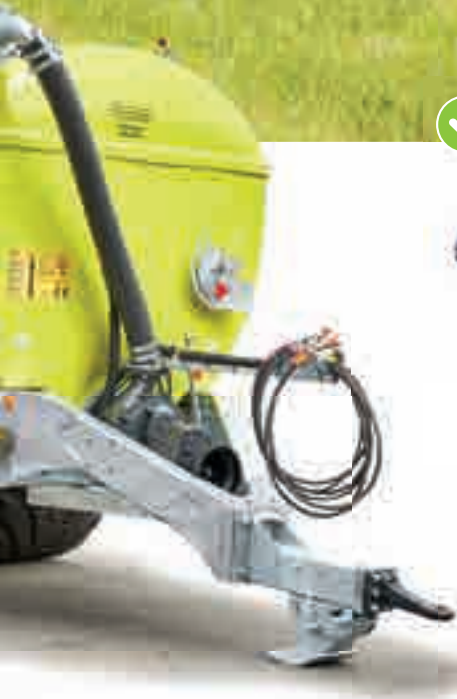
Elba centrifugal pump from Battioni, 3500 or 6500 l/min.
