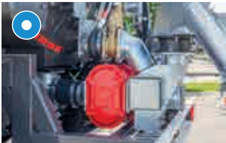
Powerful rotary piston pump from Vogelsang (model VX 186-260Q) with auxiliary suction function for emptying the slurry hose when reported as full
