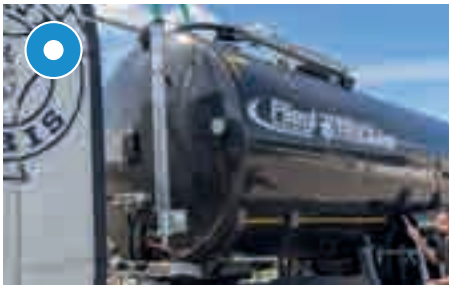
Additional fill level indicator via Plexiglas tube
